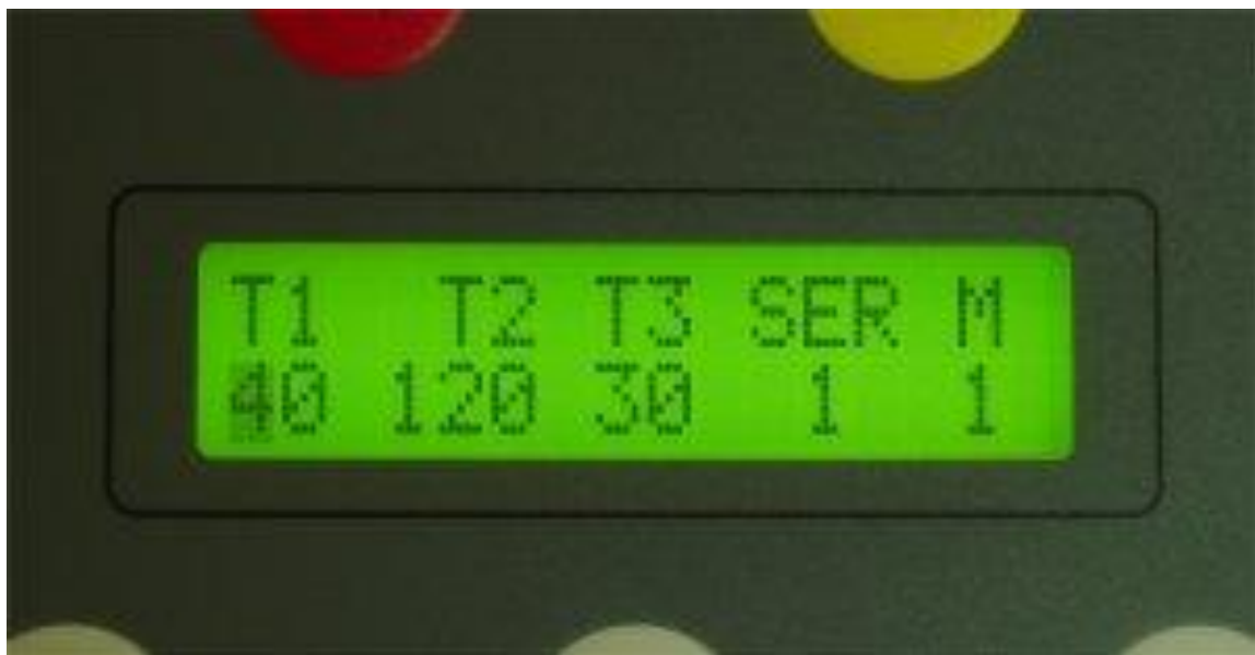
Timer Controller Display – Programming Mode
